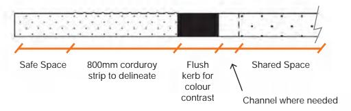
A flush corduroy strip and visually contrasting flush kerb shall run the full extents of a shared surface street to mark the transition between the Safe Space and Shared Space. For more vulnerable users a formal pedestrian crossing will still be provided within a shared surface street using the rules opposite.
